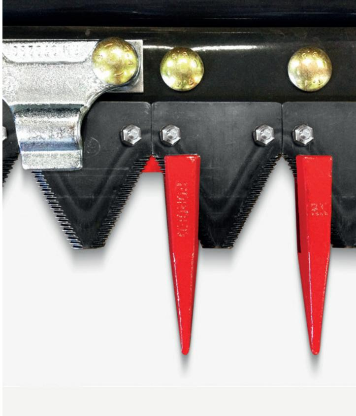
Sunstorm cutting system is specifically studied to harvest big sunflower steam. It is not a grain cutting system readjusted to sunflowers. Sunstorm has bigger knives bolted section and smoother cutting speed to guarantee long life and few vibrations.
